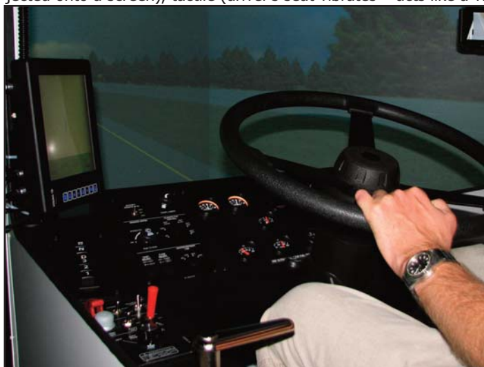
The training simulator is designed to replicate the experience of driving the bus in conditions such as may be encountered when driving on the shoulder.
