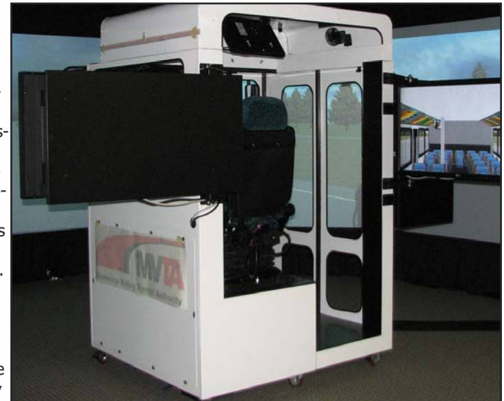
Funded by the Urban Partnership Agreement, the MVTA has acquired a training simulator to prepare drivers for using the shoulder-running BRT along Cedar Avenue.
